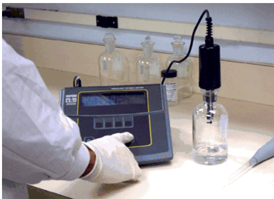
Figure: Laboratory calibration of DO meter
